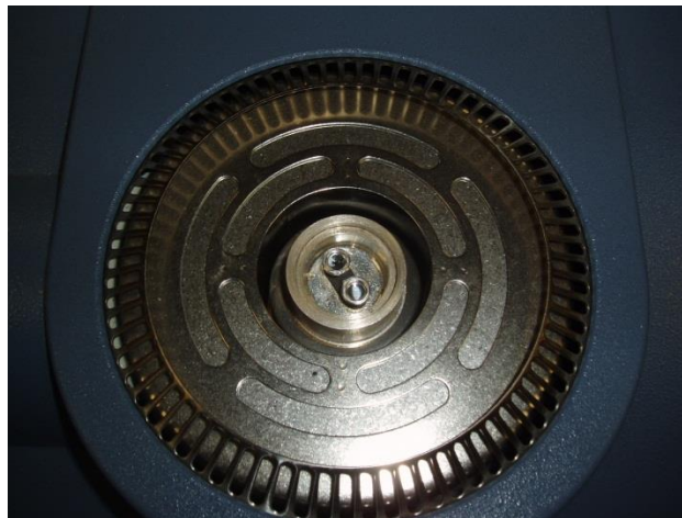
Figure 14-37. DSC sample and reference furnaces (courtesy/permission TA Instruments)
