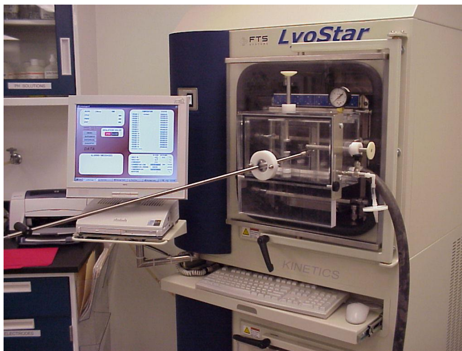
Figure 14-43. Sample thief on a development scale freeze-dryer (courtesy SP Scientific)
